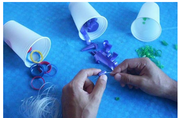
Figure 11: Making links of chain – cooking PET lines in hot water.
