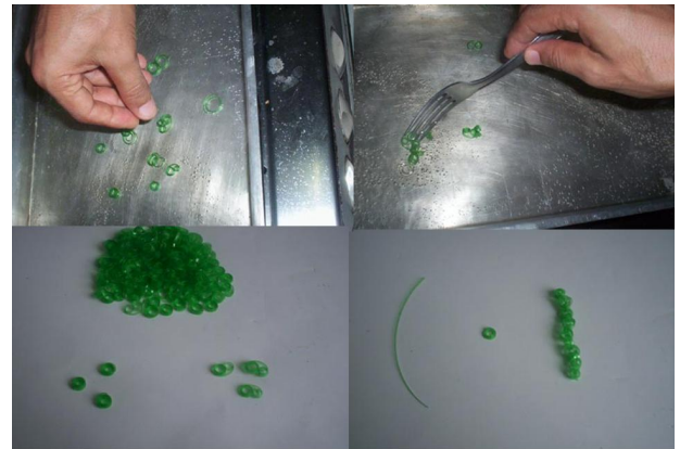
Figure 11: Making links of chain – cooking PET lines in hot water.
